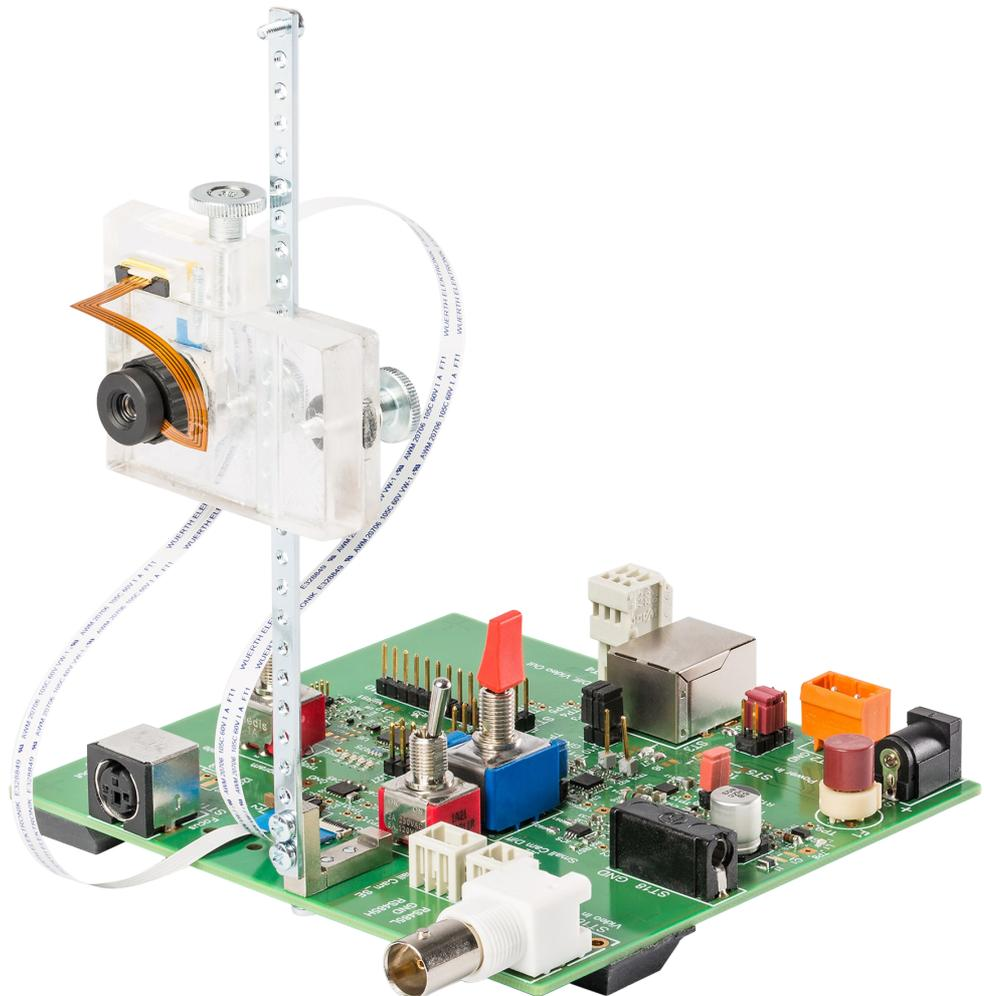
AHD-EVAL-1 prototype board with camera 21C14 from Skoopia and liquid lens optics from Varioptic (the camera with optics, connecting cables and holder are not supplied with the board)
