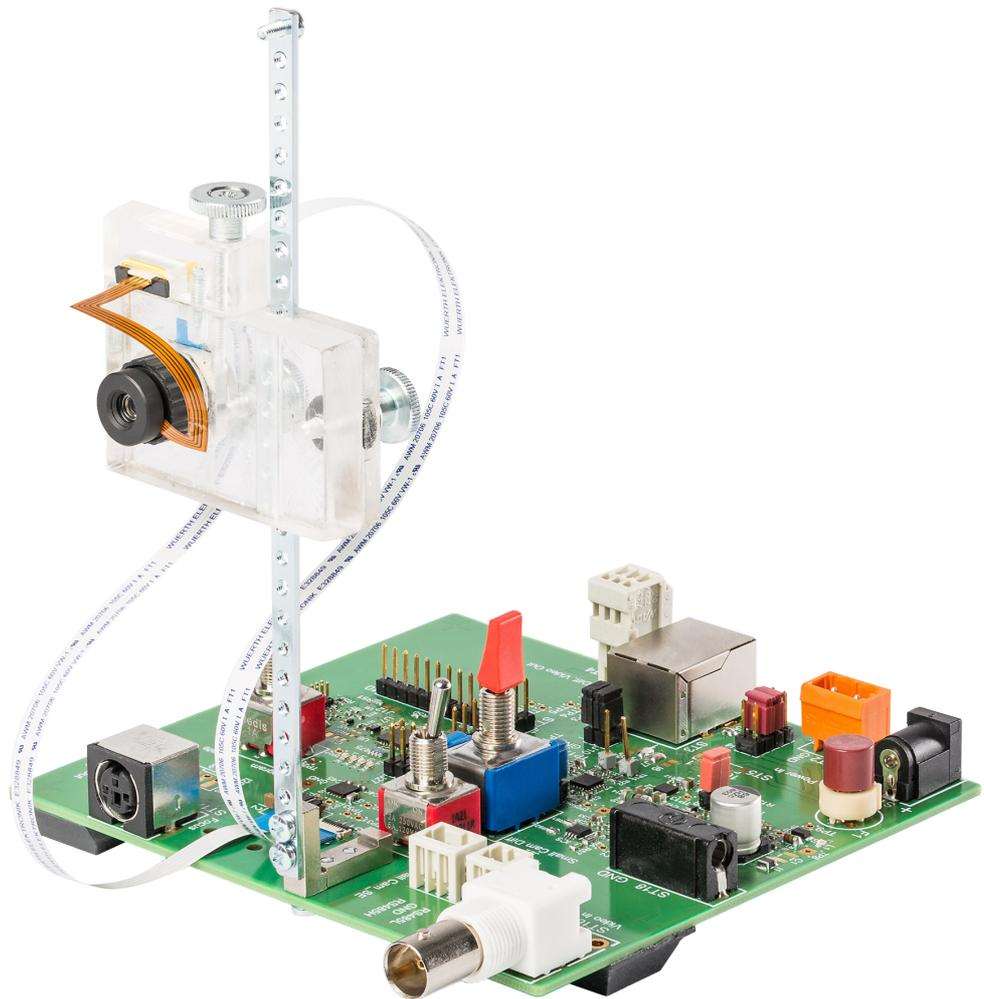
**Fig. 1 AHD-EVAL-1 prototype board with camera 21C14 from Skoopia and liquid lens optics from Varioptic**
