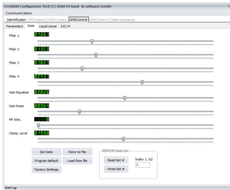
**Fig. 8 Data Tab of the AHD-VR-1 Window**
